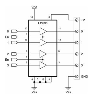
When the enable inputs are high the outputs will follow the inputs, otherwise the outputs will be in a Hi-Z state. See the L293D documentation (available separately) for additional details on use and configuration.
