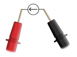
When measuring current be sure to have the leads connected as above and in the correct range, for higher currents ensure that the red lead is connected to the A 500 mA socket.
