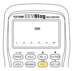
Logged data is stored to an internal Micro SD card which is accessible behind the battery cover. Data is by default recorded once per second.
