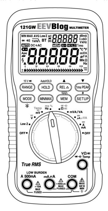
**Digital Display:** Readings are displayed on dual 4 % -digit 50,000 count LCD display. One Primary and one smaller secondary function display. The secondary function display is only used when a function that requires it is selected. A fast updating bargraph is below the main display.
