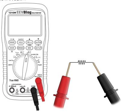
When measuring resistance select the range as shown above with the leads connected as shown above.
