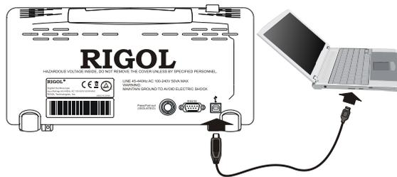
After successful connection, turn on the instrument, a dialog will guide you to install the driver of "Rigol USB Test and Measurement Device" on the PC. For VISA programming, the driver should be "USB Test and Measurement Device".
