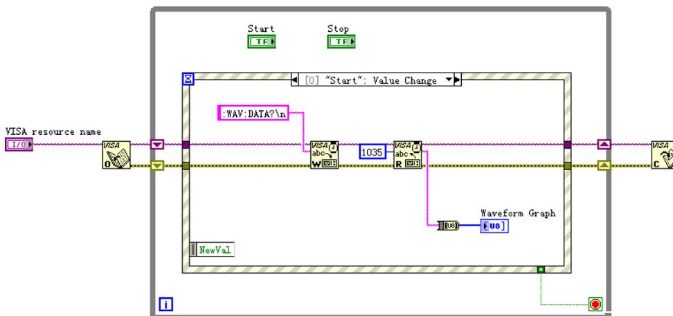
11. Adjust the style of **Front Panel** and click **"Fetch Waveform"** to get following interface. (the oscilloscope has been properly connected)
