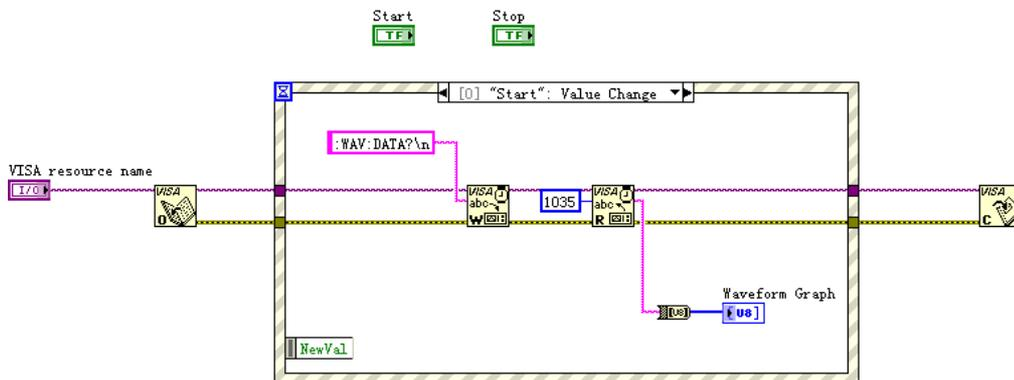
8. Right-click the **"selector label"** and choose **"Edit Events Handled by This Case"** or **"Add Event case"** to add events respectively for each button. Press **"Start"** to capture waveform and **"Stop"** to exit the program.
